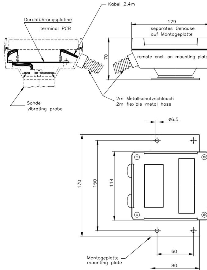
➤ Special Model HT with Temperature Insulating Tube
