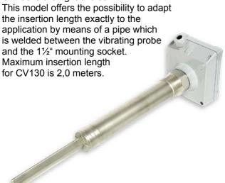
The CV130 is suitable for top mounting. Side mounting is possible for insertion lengths shorter than 1 meter and if the extension pipe is adequately supported. Connection to the container is made via thread 1 ½" DIN 2999 (equals BSPT) or NPT.
